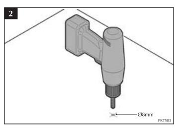
2. Remove bench and drill the two marked positions with Ø8mm hole to 50mm deep.
